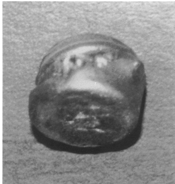
Figure 11 Cast appearance of 3Ni + Si sample ignited after pre-heating at 800°C.
